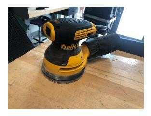
Helpful Hint: While electric sanders can speed up the finishing process, going too fast can heat up your prints and cause the material to deform and melt. Low speeds and pressure are recommended for most projects.
