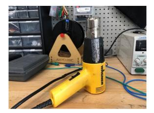
In a similar vein, heat guns are tools that are excellent for finishing prints. They can be used to reform areas that might have warped, bring color back into marred or sanded areas, and smooth out rough surfaces. Use caution as these get extremely hot!
