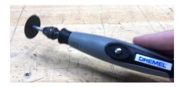
A Dremel or other small rotary tool can be used for finishing prints as well. They will often come with attachments that can help you to cut, sand and polish materials. If you take care of them, they will last a long time and can make the finishing process much easier.
