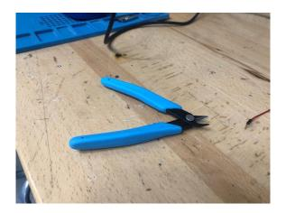
Flush cutters are one of my favorite tools. They can be used to snip off supports and when gripped lighter can be used to pull supports off in chunks. This tool will come with many printers, and it is worth holding onto.
