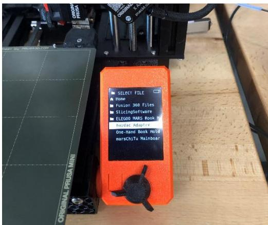
After inserting the storage device and turning your printer on, you can navigate the menu system to the file that you would like to print and start the print. Up next, I will show you the parts of a 3d printer and how they are used.
