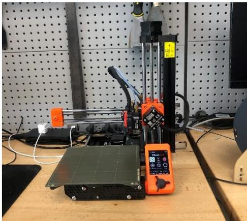
Just to get started, here is a picture of a Prusa Mini, a smaller FDM printer that is at my local makerspace. Let's go through its parts to learn about how a 3d printer works. 'FDM' stands for *fused deposition modeling*, a term that is associated with printers using a thermoplastic filament.
