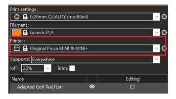
The first setting to check is the printer selection. This box will display the printer settings that have been previously downloaded. I will select the Prusa Mini from the drop down menu. The screen will then update to display the correct printer bed size.
