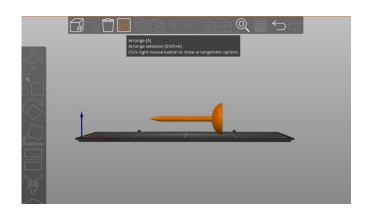
Up next, let's orientate the object on the print bed. If I positioned it golf ball side down, it would have a large base which is good, but for this print I will orient it on its side so that each layer will have a longer and stronger connection for impacts.
