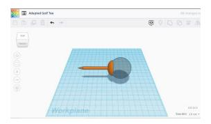
Highlighting all of the objects and selecting the 'Group' option creates an object that is roughly tee shaped. To create the divot for the ball, I will place and edit the dimensions of sphere to match the dimensions of a golf ball. I will then make it a 'hole,' align it with the top of the tee, and combine them to create a divot.
