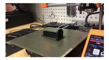
Once the print is complete, you can pull it off of the build plate. If you used supports, using tools like flush cutters and sandpaper can help to clean them off and make the print look professional.
