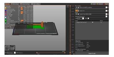
Once we are satisfied that all settings are correct, we can slice our file. This cuts the 3d object into layers that the 3d printer will follow. We can then save this as a .gcode file using the same button.
