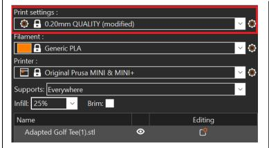
The tab on the top determines the speed and quality of our print. Faster prints tend to be slightly less refined, while high detail prints will take significantly longer. For most projects it is good to find a balance between the two, with .2 being a good starting point.
