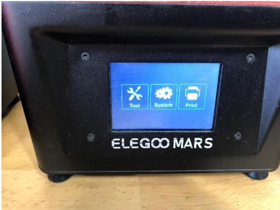
The control screen allows you to navigate through options and select which print you would like to make when you have a flash drive or other memory device inserted.
