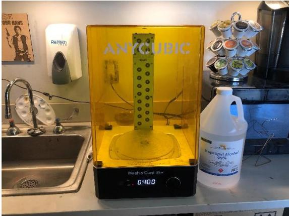
In addition to the resin printer, you may have access to a curing machine. This machine offers two purposes, the first being a washing function to remove excess resin and clean it. It also serves as a curing station, exposing the print to additional UV light to its surface.
