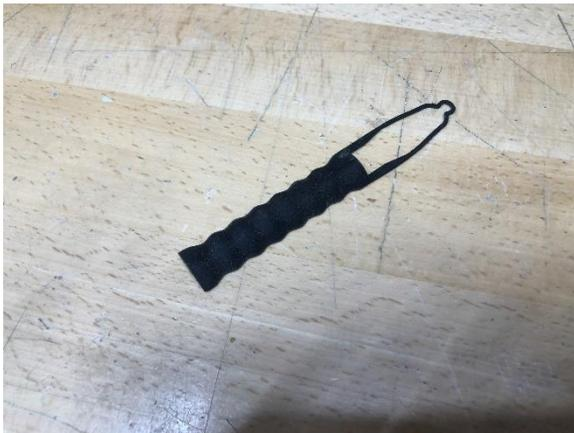
Once the print is done curing, you can finish it like you would an FDM print. You can use sandpaper to smooth any indentations from supports and paint it as desired.
