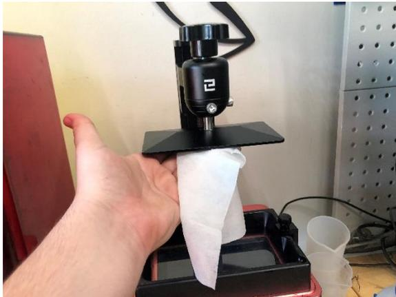
Now it is time to prepare the printer. Be sure to clean off the screen, build plate, and bottom of the resin pool with an alcohol wipe to remove any old resin or debris. If there is still resin in the pool from a previous use, use a gloved finger to stir the resin and feel for any lumps. Wipe dry with a clean microfiber cloth if needed.
