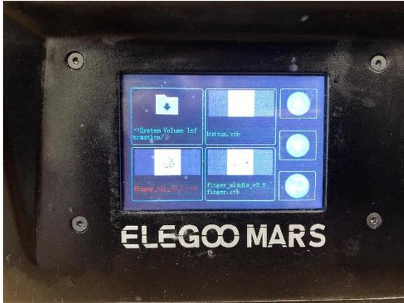
Now that the printer is prepared, we can use the menu screen to select the file that we want to print. Many printers will show a small preview image of the print that you are selecting. The printer will then run until the print is complete.
