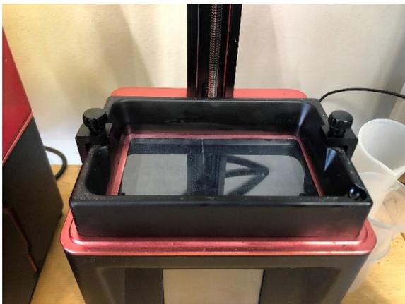
The build plate lowers itself into a pool of resin, which is held below. Different printers are able to hold different amounts of resin, determining how large of a print they can manage. The bottom of the build plate is a sheet of plastic held taught through tension. With time this material may become worn and require replacement.
