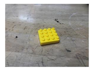
ABS is a common plastic, used in common materials like Legos. ABS is known for being strong and durable. When printing ABS, be aware that it produces fumes and should be used with a printer enclosure. ABS has a wide temperature range from around 210 to 250°C and requires a heated bed to print on.
