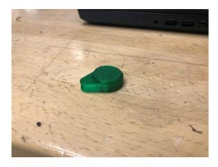
PETG is a form of plastic that is similar to the plastic that is used in soda bottles, altered for use in 3d Printers. It has a relatively high printing temperature (220 – 250°C), although many printers can accommodate it in the low range. PETG is a very durable material with okay flexibility. A heated bed is necessary, and you may consider using painters' tape, hairspray or a glue stick on the print bed to help with adhesion.
